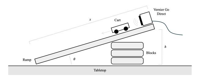
1. Spend a little time designing your experimental setup. Measure the total height and total length of the ramp. Record these values in an Excel (or equivalent) spreadsheet.
